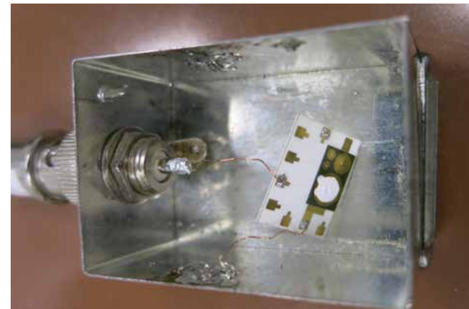
SiC detector with a diameter of 8 mm and an applied 6LiF conversion layer connected to the testing spectrometric chain for thermal neutron detection.
