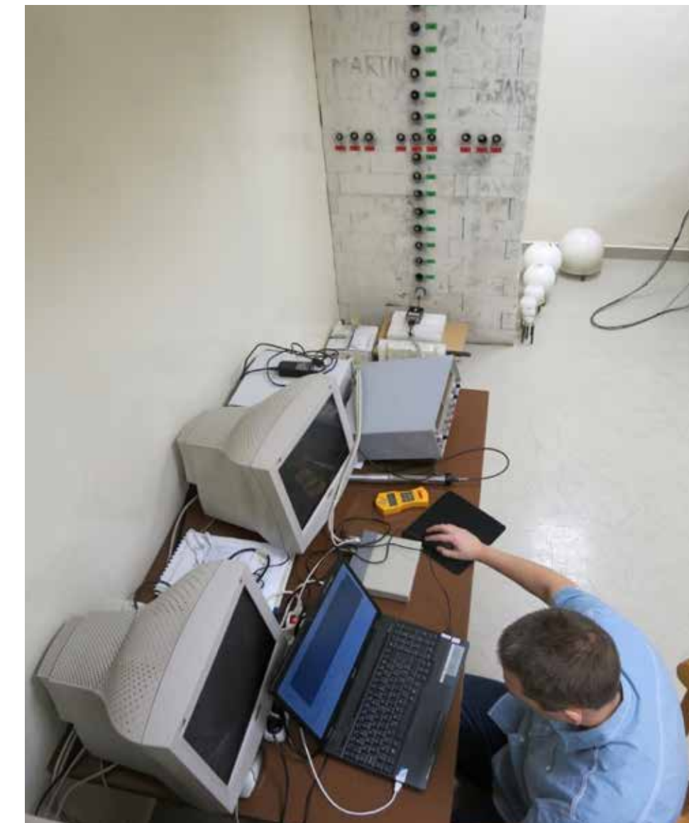
Measuring the thermal neutrons produced by stopping fast neutrons from the ^{239}\text{PuBe} neutron source at FEEIT SUT in Bratislava. The SiC detector with a 6LiF conversion layer is placed directly in the shielding structure of the neutron source.
