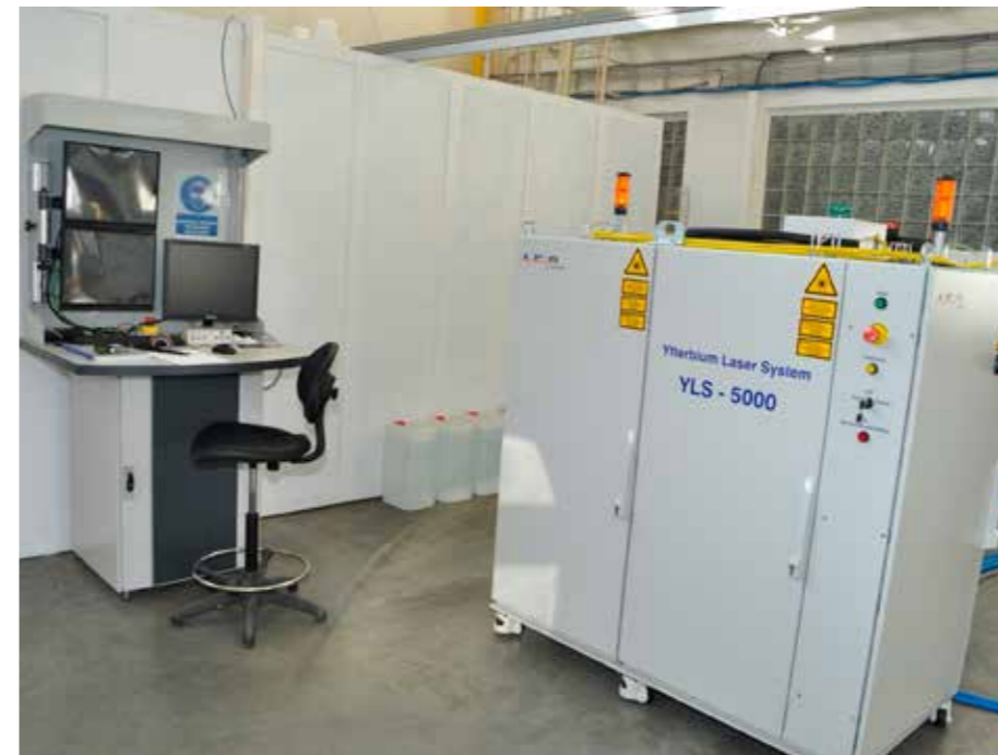
Fig. 1 / The experimental laser work station with the IPG YLS 5000 fibre laser for welding aluminium and magnesium alloys.
